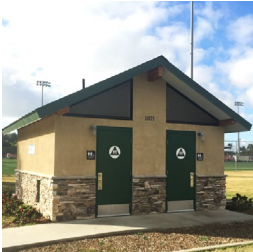
Restroom (Alt. 4) Manufacturer: Romtec Model: 2024 - Double Restroom Design: 2-single occupant, mech. & storage Color/Material: Coordinate with preferred shelter and site furnishing standards. Size: 16'8" x 16'8" + 5' concrete walk Cost: $60k - 100k (design, material) + $90k - 150k (install)
