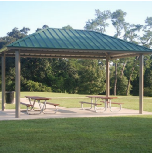
Shelter (Alt. 1) Manufacturer: Poligon Product: Hip Roof Rectangle Model: RAM 16x24 Color/Material: Coordinate with preferred shelter and site furnishing standards. Roof Pitch: 6:12 Cost: $28.3k (includes installation) Capacity: 6 picnic tables
