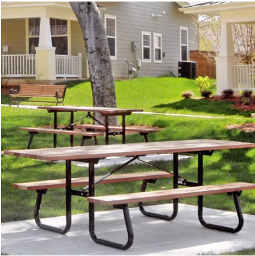
Picnic Table Manufacturer: Victor Stanley (Homestead Collection) Model: ST-5 6'-0" long table, wood (IPE) slats, surface mount tabs, tables anchored at shelters Steel Color: Black powder coat at 8-10 mils thick Cost: $4,000
