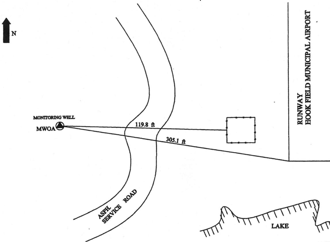
The mark is a NGS Standard Control Disk, set in a large structure (monitoring well), stamped "MWO A 1995", in the Hook Field Municipal Airport. The mark is located 305.1 feet from the southwest corner of the runway and 119.8 feet from a fenced area to the east.
