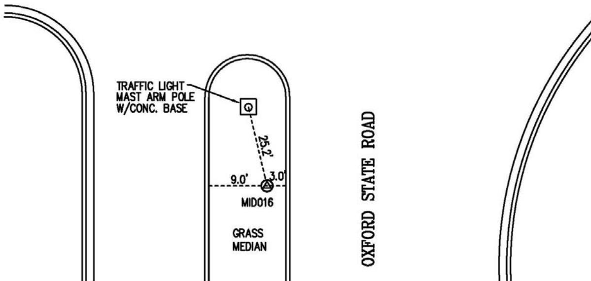
The mark is a concrete monument with a bronze cap located in the median of Oxford State Road, approximately 90 feet east of the centerline of Cincinnati-Dayton Rd.. The mark is located 25.2 feet from a traffic light mast arm pole to the west, 3.0 feet from the north back of curb of median and 9.0 feet north of south back of curb of median.
