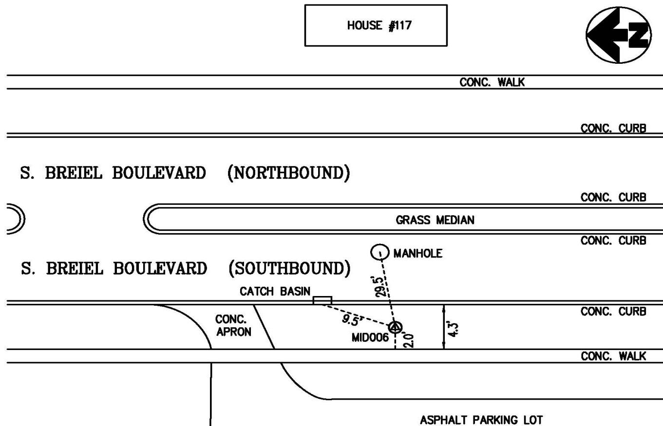
The mark is a concrete monument with a bronze cap located along the west side of Breiel Boulevard, approximately 0.12 miles north of the centerline of Batsey Drive. The mark is located 2.0 feet east from the face of a concrete walk, 9.5 feet from a catch basin to the northeast and 29.5 feet from a manhole to the east.
