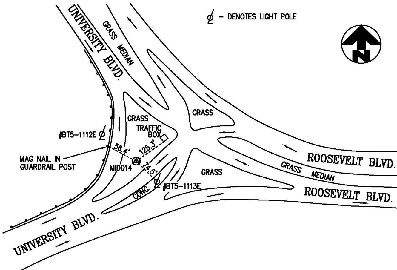
The mark is a concrete monument with a bronze cap located in the median of the University Blvd. / Roosevelt Blvd. interchange. The mark is located 74.5 feet from a light pole (BT5-1113E) to the southeast, 125.3 feet from a traffic box to the northeast and 56.4 feet from a guardrail post with a Mag Nail (being the first guardrail post south of light pole (BT5-1112E)).
