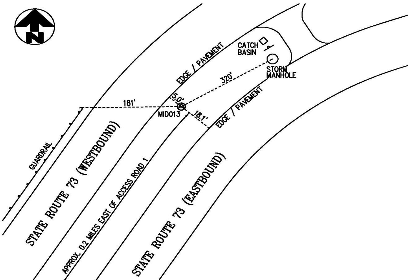
The mark is a concrete monument with a bronze cap located in the median of State Route 73, approximately 0.2 miles east of Access Drive 1. The mark is located 5.0 feet south from the easterly edge of pavement of the west bound lane, 18.1 feet north from the westerly edge of pavement of the east bound lane and 320 feet from a storm manhole to the east.
