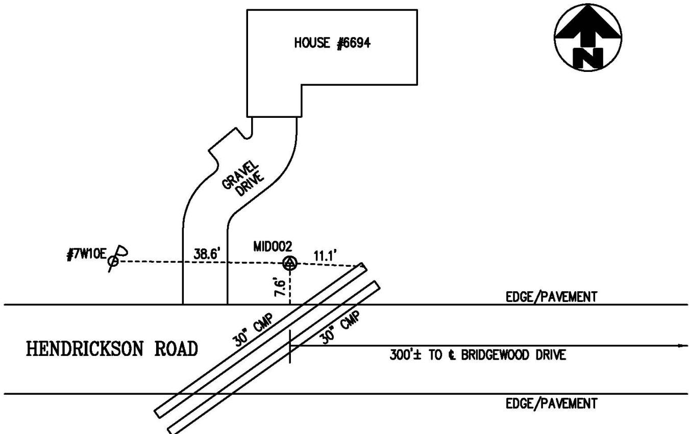
The mark is a concrete monument with a bronze cap located along the north side of Hendrickson Road, approximately 300 feet west of the centerline of Bridgewood Drive. The mark is located 7.6 feet north of the north edge of pavement and 11.1 feet west of the north end of a 30" corrugated metal pipe.
