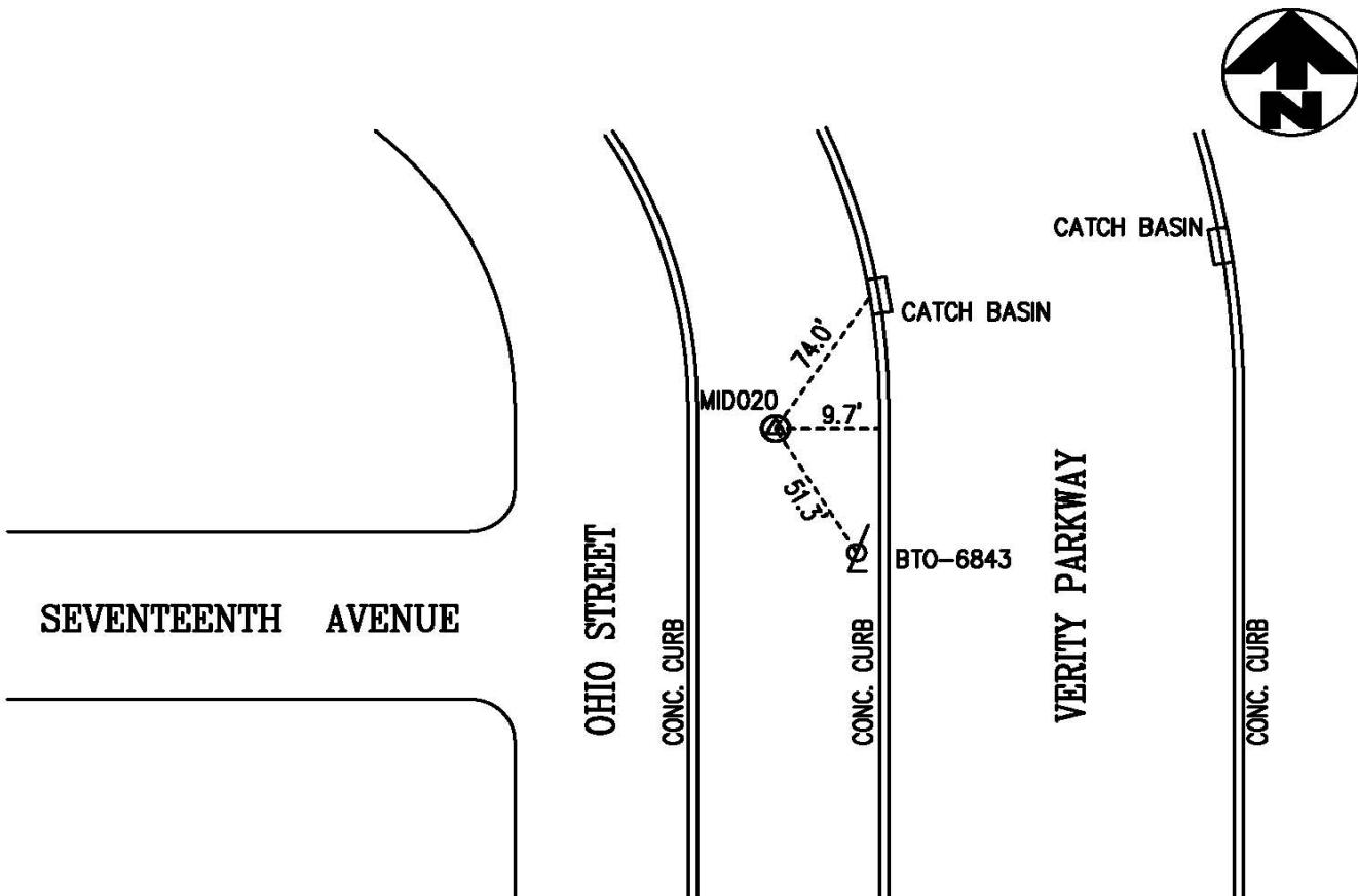
The mark is a concrete monument with a bronze cap located in the median between Verity Parkway and Ohio Street, just north of Seventeenth Avenue. The mark is located 74.0 feet from a catch basin to the northeast, 9.7 feet from the west back of curb of Verity Parkway and 51.3' from a power pole to the southeast (BTO-6843).
