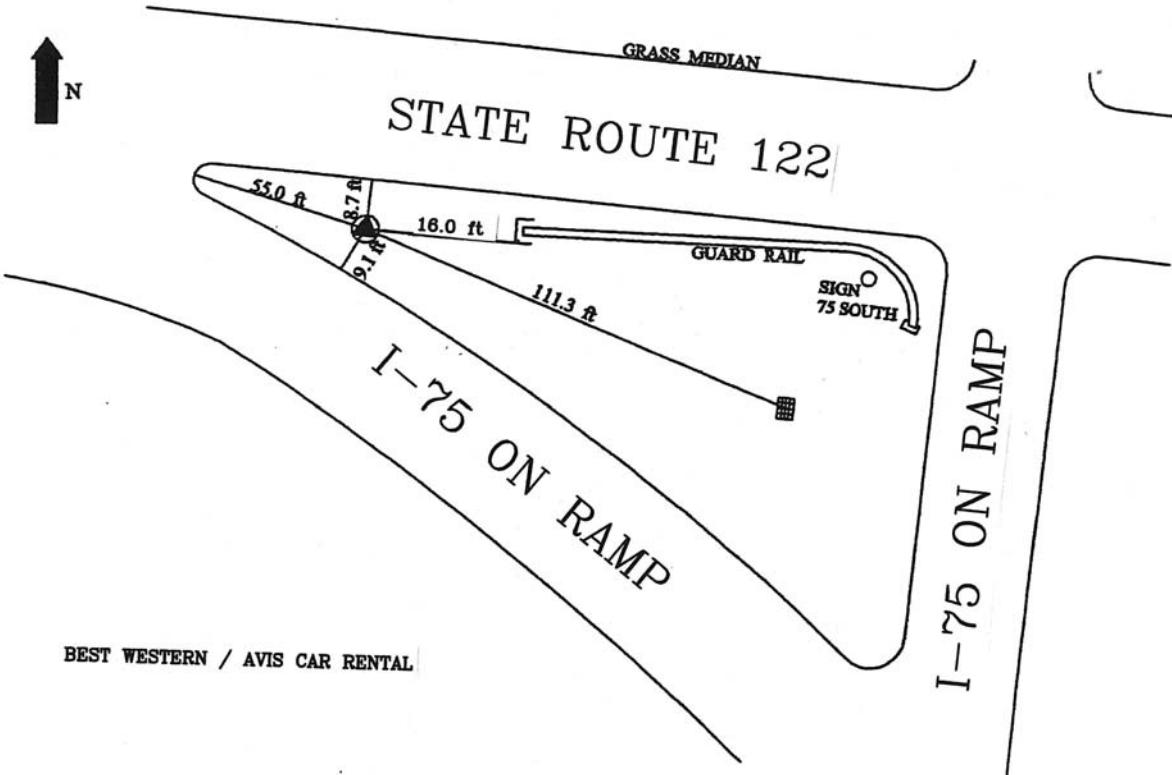
The mark is a concrete monument with a brass disk "Butler County Engineers Ref. Monument" stamped "99FC72A" located on the south side of State Route 122 in the median of the entrance ramp to southbound Interstate 75. The mark is located 8.7 feet south of the south edge of pavement of State Route 122, 9.1 feet north of the north edge of pavement of Interstate 75 entrance ramp and 16 feet from the end of a guardrail located to the east.
