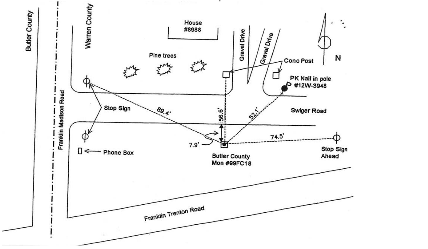
The mark is a concrete monument with a brass disk "Butler County Engineers Ref. Monument" stamped "99FC18" located on the south side of Swiger Road, east of the intersection of Franklin Madison Road and Swiger Road. The mark is located 7.9 feet south of the south edge of pavement and 52.1 feet from a power pole (12W-3948) to the northeast.
