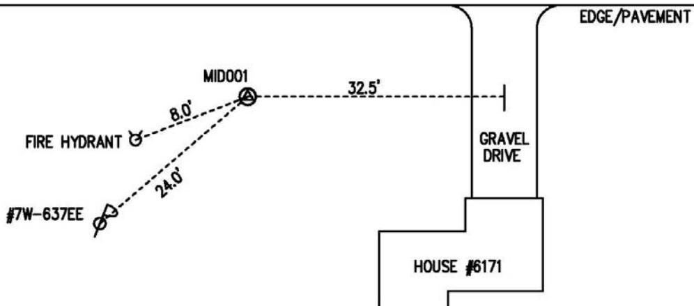
The mark is a concrete monument with a bronze cap located along the south side of Hendrickson Road, approximately 0.16 miles east of the I-75 overpass. The mark is located 32.5 feet west of the centerline of a gravel drive to #6171 Hendrickson Road and is also located 8.0 feet northeast of a fire hydrant.
