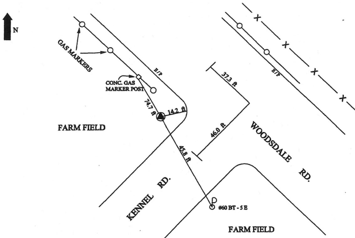
The mark is a concrete monument with a brass disk "Butler County Engineers Ref. Monument" stamped "99FC68" located on the northwest corner of Woodsdale Road and Kennel Road. The mark is located 46.0 feet southwest of the centerline of Woodsdale Road, 37.3 feet northwest of the centerline of Kennel Road and 45.8 feet from a power pole to the southeast (60 BT-5E).
