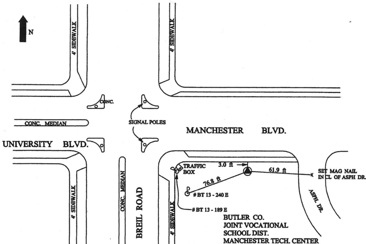
The mark is a concrete monument with a brass disk "Butler County Engineers Ref. Monument" stamped "99FC74" located on the southeast corner of the intersection of Manchester Road and Breil Boulevard. The mark is located on the south side of Manchester Road, 3.0 feet south of a concrete sidewalk and 76.8 feet from a power pole (BT13-240E) to the southwest.
