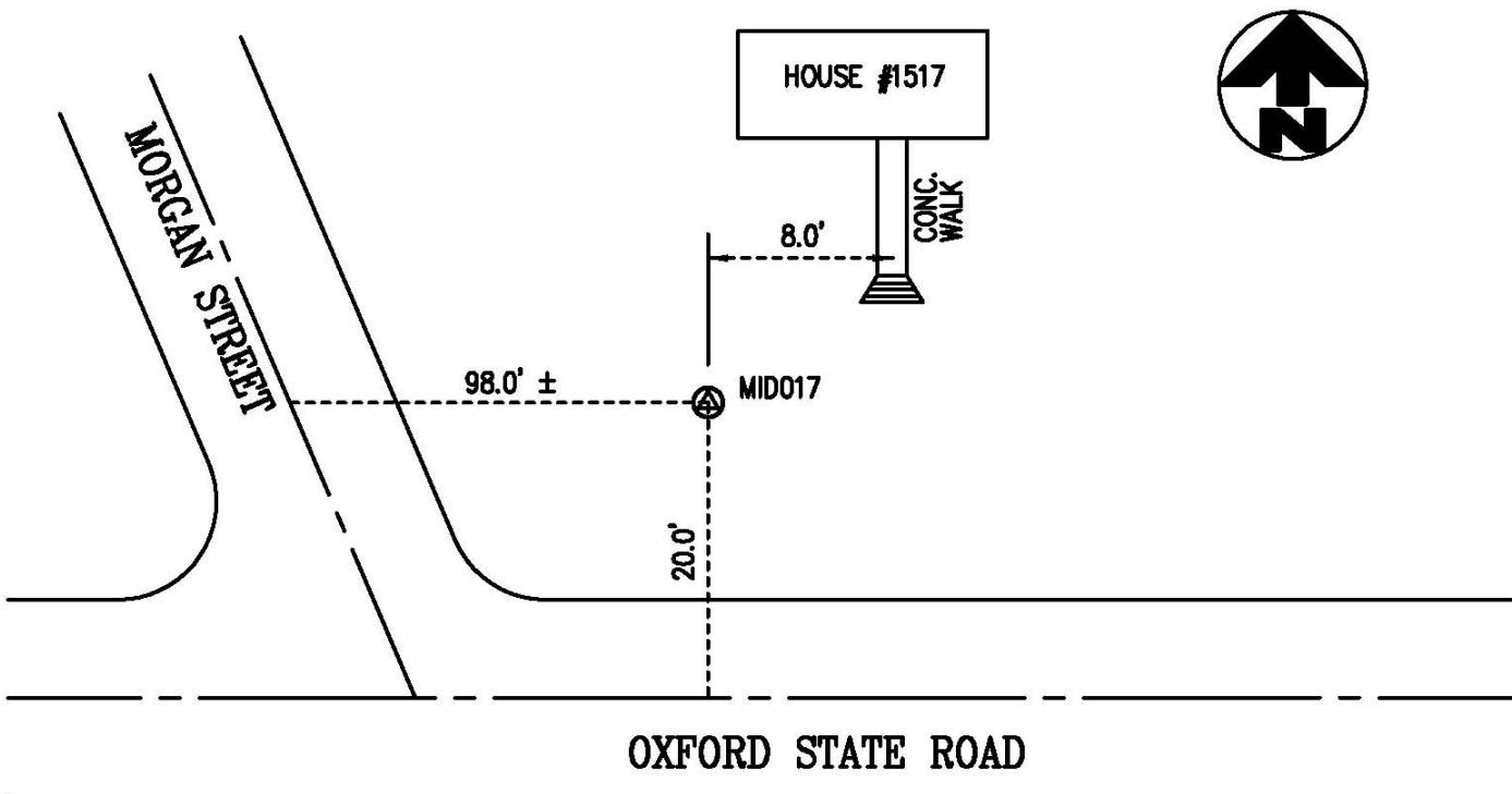
The mark is a concrete monument with a bronze cap located on the north side of Oxford State Road, approximately 98 feet east of the centerline of Morgan Street. The mark is located 20.0 feet from the centerline of Oxford State Road and 8.0 feet west of the southerly extension of the centerline of a concrete walk to house #1517 Oxford State Road.
