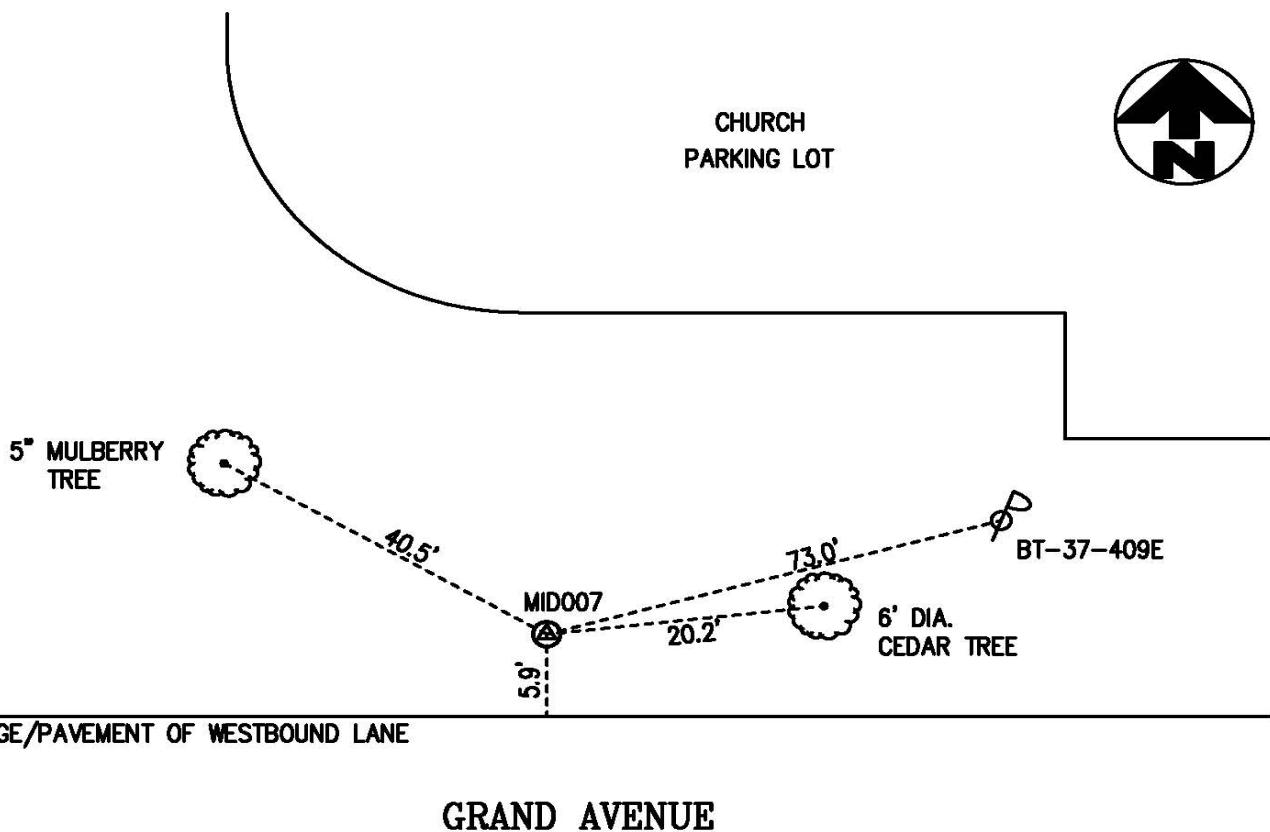
The mark is a concrete monument with a bronze cap located along the north side of Grand Avenue, approximately 0.13 miles west of the centerline of Marshall Road. The mark is located 5.9 feet north from the north edge of pavement of the west bound lane, 40.5 feet from a 5" tree to the northwest and 73.0 feet from a power pole (BT-37-409E) to the northeast.
