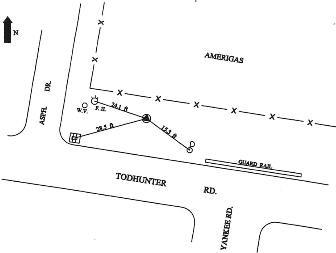
The mark is a concrete monument with a brass disk "Butler County Engineers Ref. Monument" stamped "99FC67" located on the north side of Todhunter Road, west of the intersection of Todhunter Road and Yankee Road. The mark is located 24.1 feet from a fire hydrant to the west and 15.3 feet from a power pole to the southeast.
